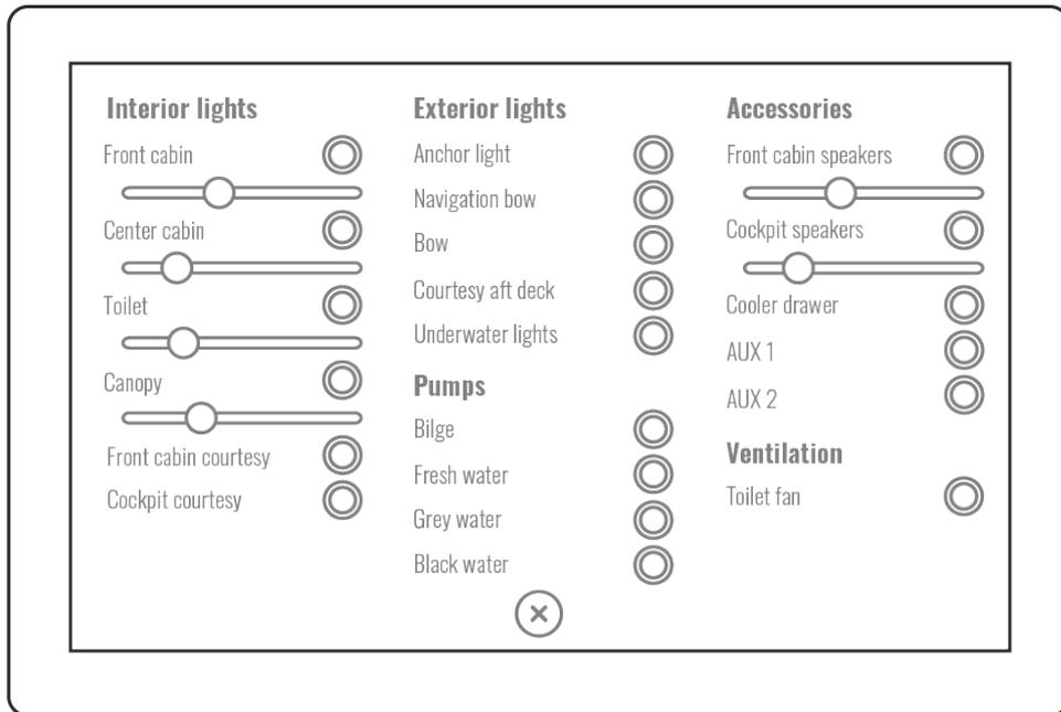
You can control boat's lighting, pumps and other accessories on Q system's Boat Controls application. The app contains simple on/off controls for each appliance and sliders for some appliances, e.g. stereo. Note that Boat Controls are only available in your boat if it has the Q Switch installed.
