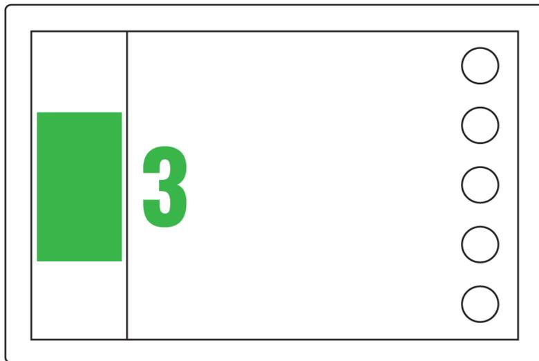
3. **Motor data** Sidebar's middle part displays engine data. Tap on the field to open dashboard.
