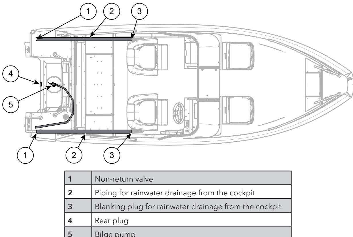
Bilge pumps or the ends of suction tubes are located as close to the baseboard as possible. It is, however, natural that the bilge always contains a small quantity of water that the bilge pump cannot remove.
